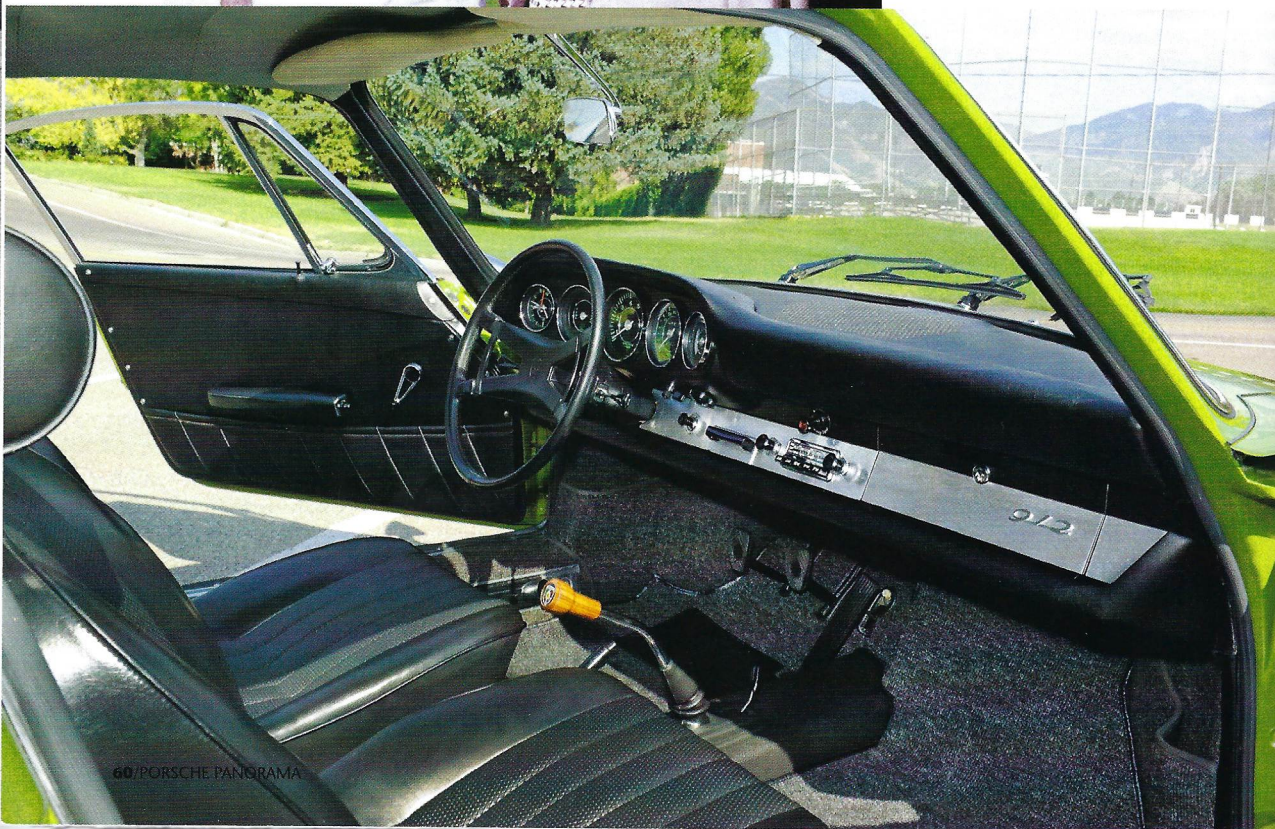
Virtually all of the Porsche, born a 912, has been modified to meet Jerry's vision of the car he wanted. A five-gauge 911 dash has been added to the interior.
