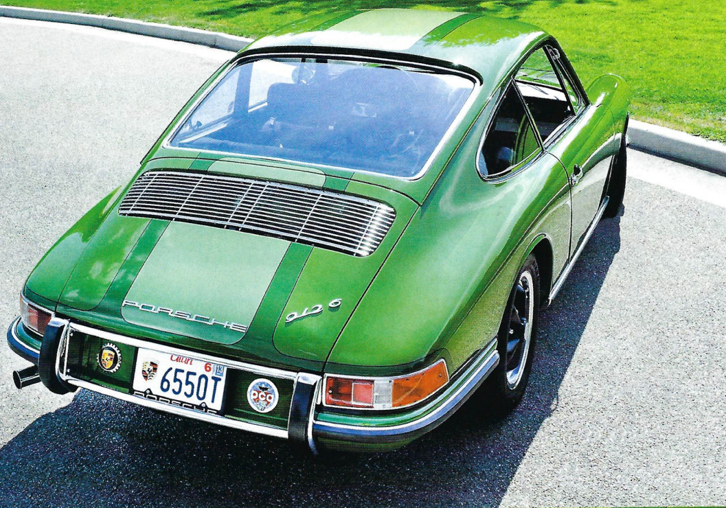
The rear is stock except for the addition of the "6" to the 912 insignia, hinting at the six-cylinder engine under the deck.
