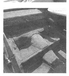
Comfort waived to save weight: manual window cranks, seats and heater controls. Folding rear seats have been eliminated.
